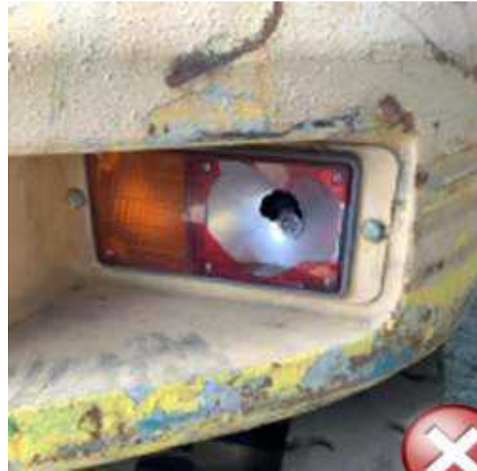
Damaged Signal Light
