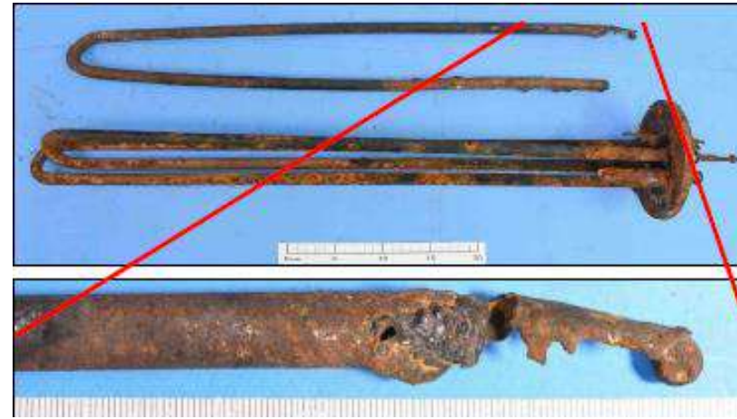
Post-explosion view of spoiled heater, likely to be heater #1, that was replaced on 8 August 2020
